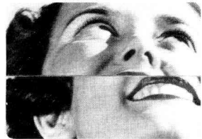
The halves of the image, as seen through the range finder, are split and out of alignment here as the lens is focused for a distance shorter than that from camera to subject.
